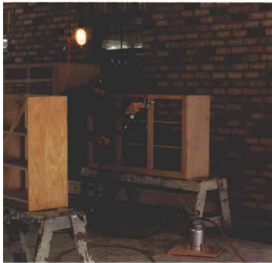
For finishing cabinets (above), Papa prefers to use a conventional spray gun because it is easier to control than the airless variety. Papa has modified this rig by adding the 2-qt. pressure cup held fast by the portable wooden base on the floor. Note the trouble light; Papa shines it on surfaces to check for sags in the finish. Using a spray gun with a siphon cup (below), the author sprays Deft on a cabinet door. The back of the door has already been finished, and he is now spraying the rails and stiles from both sides to get thorough coverage.
