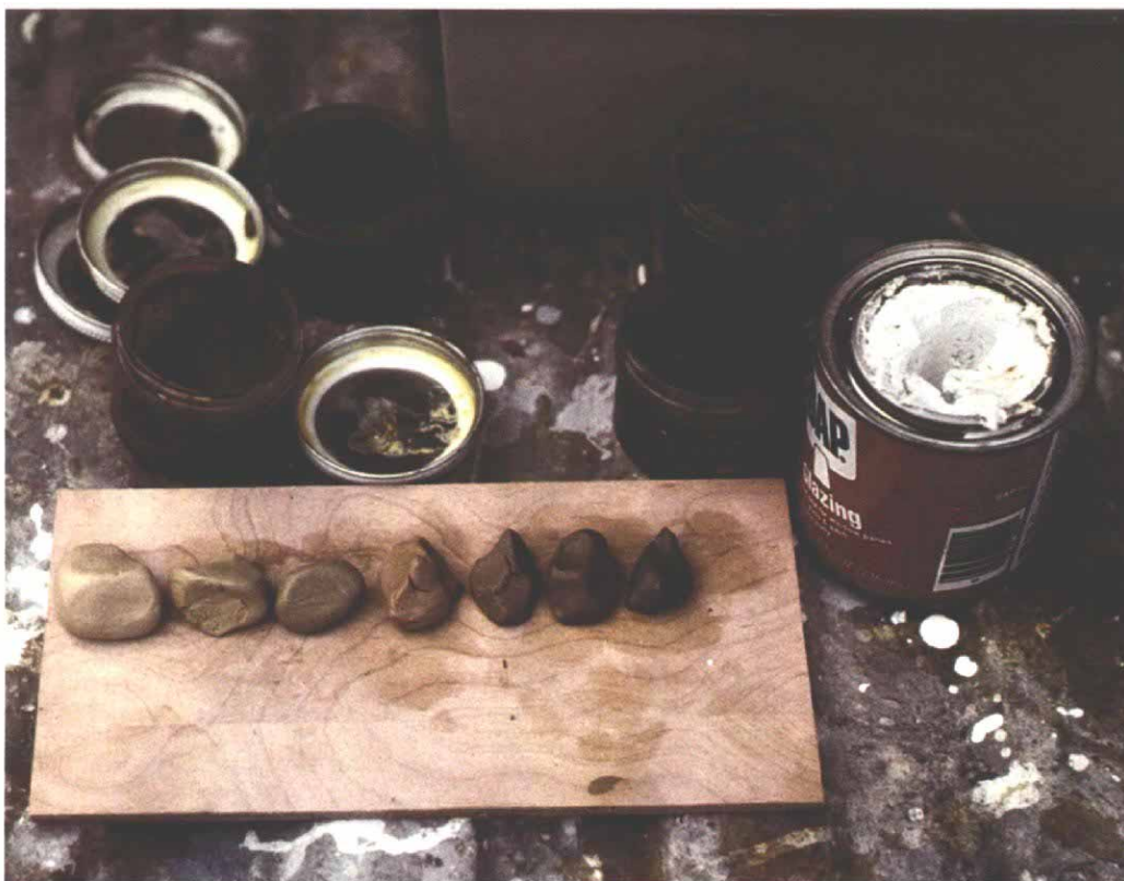
It takes a lot of colors to match a variegated material like wood. Papa begins with Color Putty in a variety of tones and modifies them with white glazing compound and universal paint pigment to match the wood in question. For recipes to match common woods, see the chart on p. 78.
