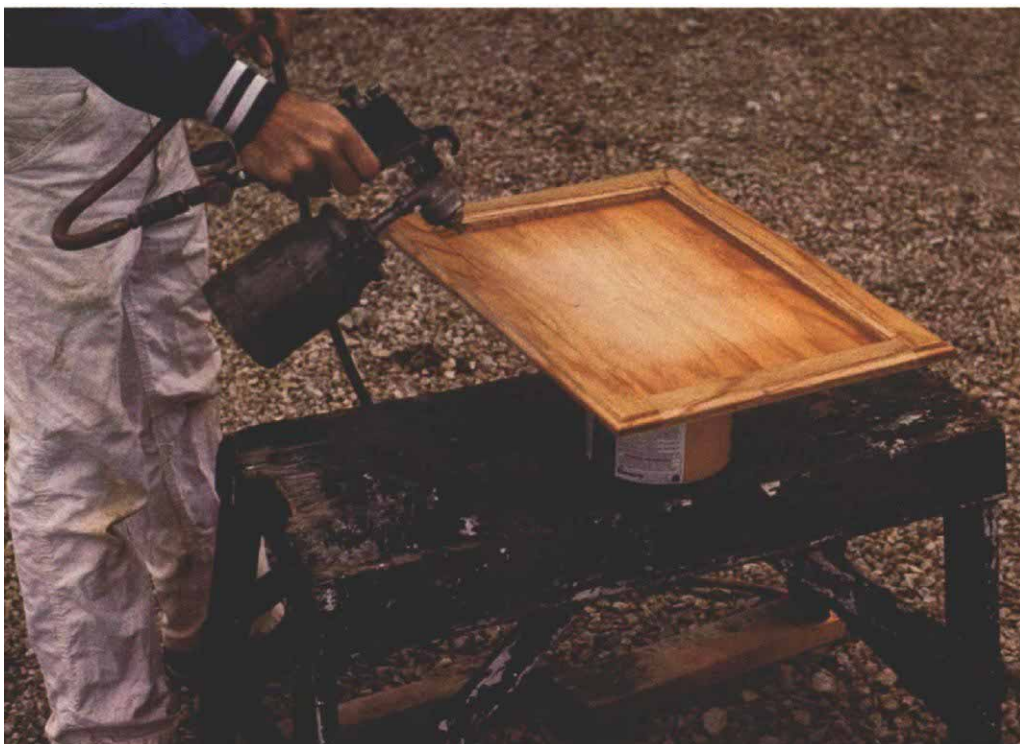
For finishing cabinets (above), Papa prefers to use a conventional spray gun because it is easier to control than the airless variety. Papa has modified this rig by adding the 2-qt. pressure cup held fast by the portable wooden base on the floor. Note the trouble light; Papa shines it on surfaces to check for sags in the finish. Using a spray gun with a siphon cup (below), the author sprays Deft on a cabinet door. The back of the door has already been finished, and he is now spraying the rails and stiles from both sides to get thorough coverage.
